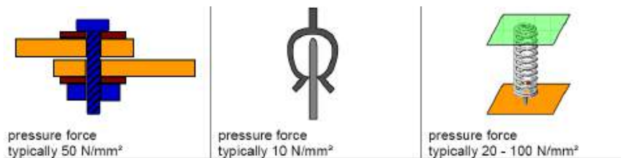
Figure 2.5.7 Comparison of contact pressures of detachable electrical connections (from left to right: screw, plug-in, spring contact)
