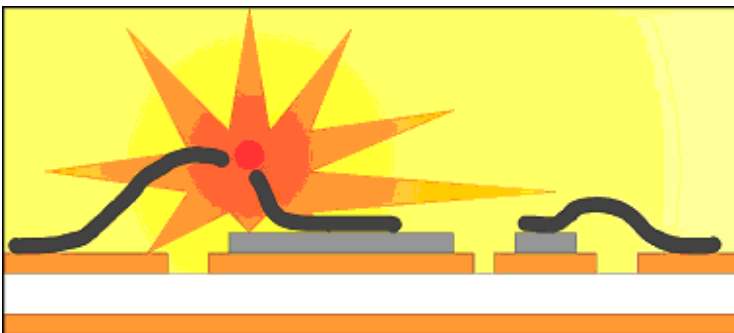
Figure 2.6.7 Possible voltage flashover to the insulated temperature sensor if a bond wire melts as a result of a fault
