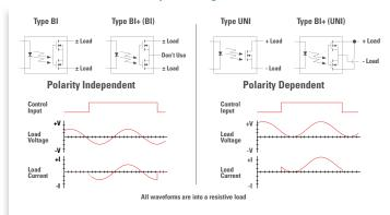
Type BI relays conduct load current in both directions.
