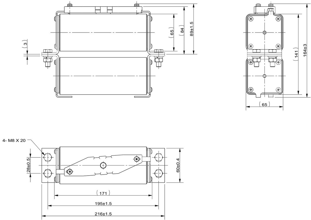
170M2044 and 170M2045 - Parallel Double Slot Tag
