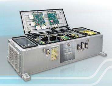
KONTRAC PN25DC is used as the auxiliary power supply converter in tramway vehicles. It converts 600 VDC or 750 VDC line voltage into three-phase AC voltage intended for supplying of tramway's air-conditioning unit.
