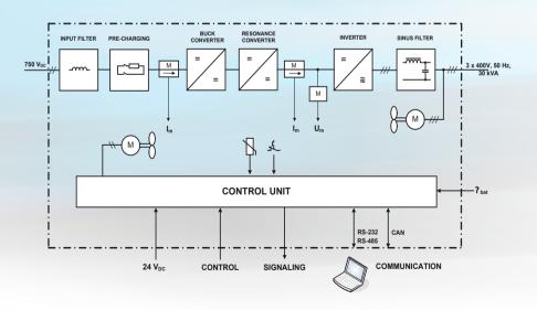
Block diagram of the converter
