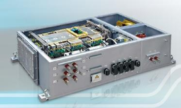
KONTRAC GP170DC converts 600 VDC or 750 VDC line voltage into propulsion power to control and drive asynchronous traction motors on tramway vehicles. The converter supplies two asynchronous traction motors connected in parallel. The electrical motor drive operates in two modes: traction mode and braking mode.
