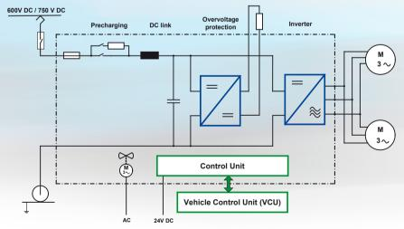
Block diagram of the converter
