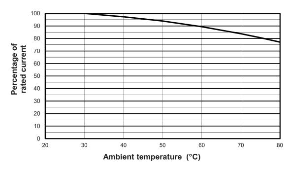
(The ambient temperature is that local to the fuse link)
