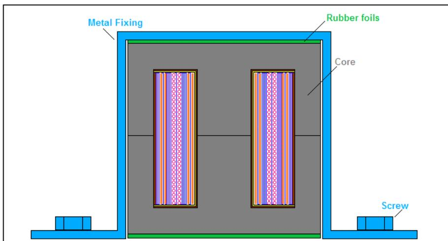
Several materials are available on the market, such as thermo-conductive rubber foils which help to avoid mechanical stresses on the cores and to improve, at the same time, the transfer of the heating due to core losses.
