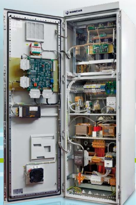
KONTRAC PN30AC is a trackside auxiliary power supply converter fed by 25 kV, 50 Hz overhead line. It is used in order to supply various loads inside the substation facilities (power supply for integrated lighting and information systems, railway signaling and protection systems, etc.). Overhead line might generate spikes, sags and surges caused by the current drawn from locomotives. Those are likely to damage the input stages of conventional converters.
