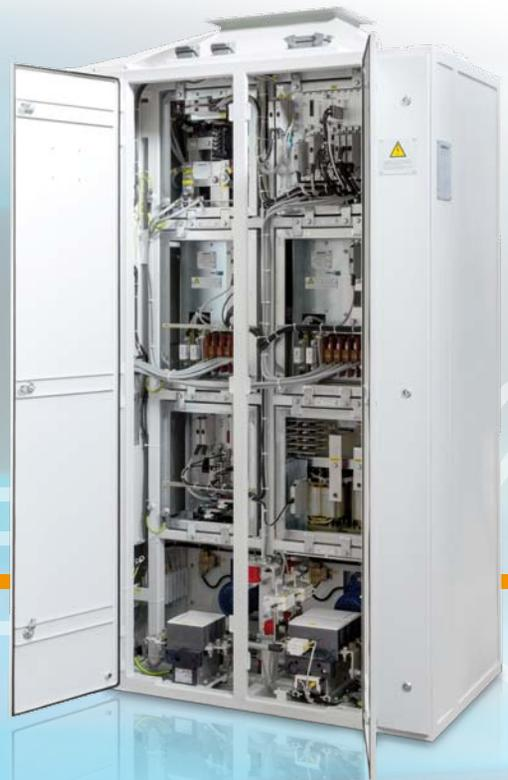
KONTRAC PN110AC is used as the auxiliary power supply converter in multiple unit trains. It is fed from a dedicated winding of the main transformer and supplies stabilized voltages to electrical loads. The converter has two three-phase outputs and one DC output. Its input current is nearly sinusoidal and its fundamental harmonic is in phase with the input voltage.
