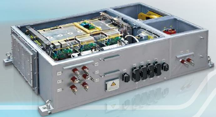
KONTRAC GP170DC converts 600 Vdc or 750 Vdc line voltage into propulsion power to control and drive asynchronous traction motors on tramway vehicles. The converter supplies two asynchronous traction motors connected in parallel. The electrical motor drive operates in two modes: traction mode and braking mode.
