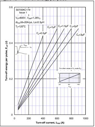
Figure 14 – Typical turn-off energy per pulse
