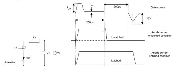
Diagram 4, Latching test circuit and waveforms.
