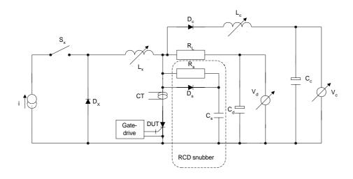
Diagram 10, Turn-off test circuit.
