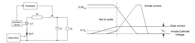
Diagram 7, Gate trigger circuit and waveforms.
