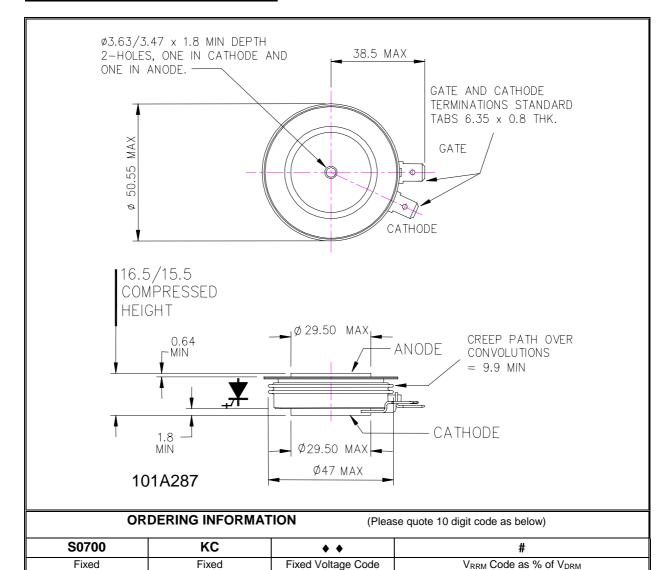
Typical order code: S0700KC17G – 1700V V<sub>DRM</sub>, V<sub>RRM</sub>=65%V<sub>DRM</sub> (1105V), 16.5mm clamp height capsule.
