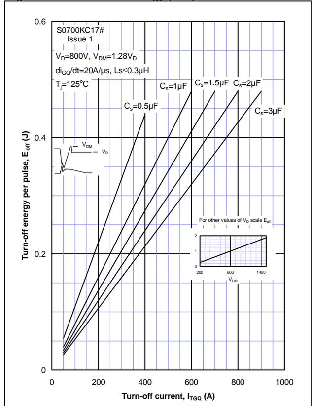
Figure 14 – Typical turn-off energy per pulse
