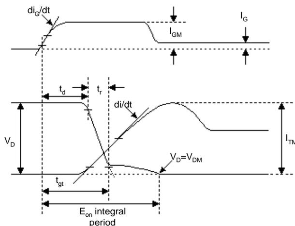
Diagram 9, Turn-on wave-diagrams.
