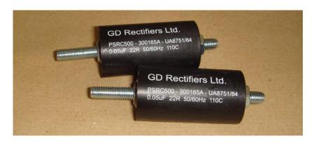
GD RECTIFIERS has developed a range of encapsulated Transient Dv/Dt Snubber Networks for protection of semiconductor components against fast rising voltage spikes that may exceed the Dv/Dt rating of the SCR's. In addition to voltage protection the modules also assist in latching SCR's used for low-level Inductive load currents. The PSRC500 and PSRC760 Stud mounted and connected modules give a rugged design suited to discrete device assemblies.
