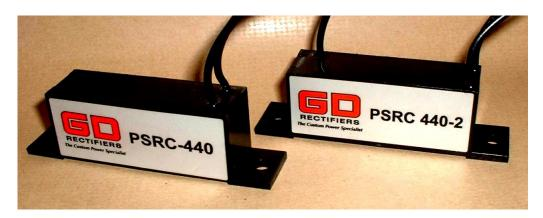
GD RECTIFIERS has developed a range of encapsulated Transient Dv/Dt Snubber Networks for protection of semiconductor components against fast rising voltage spikes that may exceed the Dv/Dt rating of the SCR's.
