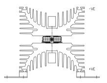
CONNECTIONS M8 CHANNELS. FIXINGS 8 x M6
