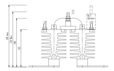
CONNECTIONS M6 FIXING 4 x M6 CLEAR
