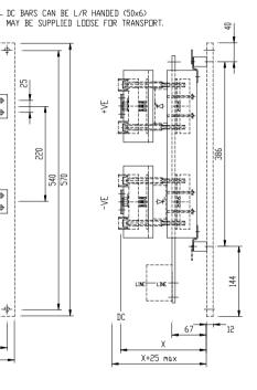
FIXINGS M8 AC/DC CONNECTIONS 2\*M8 (FUSE 32TTF M10 / 33TTF M12) G/K LEADS 600 mm
