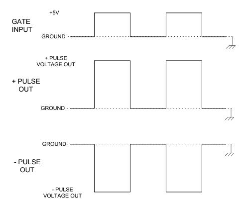
Output Pulse Configuration With Non-Inverted Gate Selected
