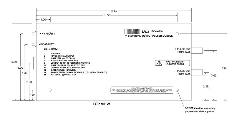
PVM-4210 Mechanical Dimensions And Mounting Hole/Connector Locations
