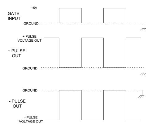
**Output Pulse Configuration With Inverted Gate Selected**
